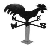
**Wind vane**: Instrument that shows the direction the wind is blowing
